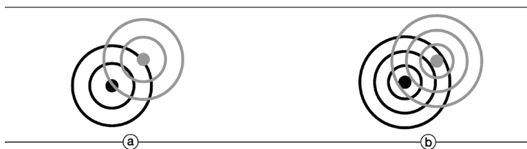
Figure 4.2 (a) The outgoing wave (black) interferes constructively with the incoming wave (gray); (b) Changing the wavelength, the interference is now destructive.
