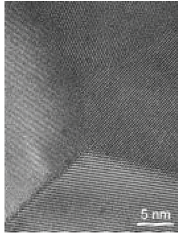
Figure 4.11 High-resolution transmission electron microscopy of grain boundaries in a sample of YSZ with an average grain size of 120 nm. Reprinted from Prog. Mater. Sci. , 51, Guo and Waser, Electrical properties of the grain boundaries of oxygen ion conductors: Acceptor-doped zirconia and ceria, pp. 151–210, Copyright 2006, with permission from Elsevier [23].
