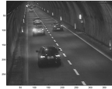
Figure 9.4: Non-perpendicular imaging system geometry.
