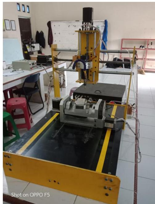
Gambar 4.31 Merakit *Rotary Table A/B*
