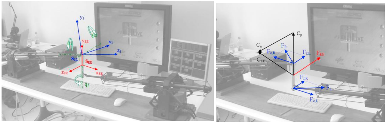
Figure 3: (Left) Handle frame and rotation angles of gimbals. (Right) Forces and torques on the handle
