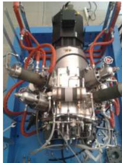
Fig. 8: Photo of the High Energy Density Stirling engine proposed by FBK
