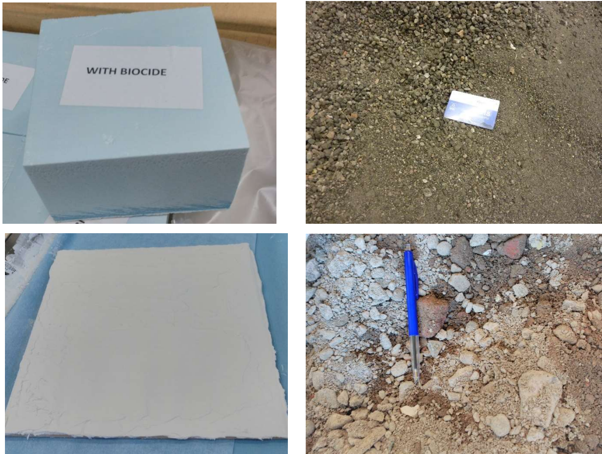
Figure 1. Starting materials for the methods CEN/TS 16637-2 and 16637-3. From top to down, and from left to right: (a) organic render, (b) sealant, (c) asphalt aggregate and (d) recycled aggregate
