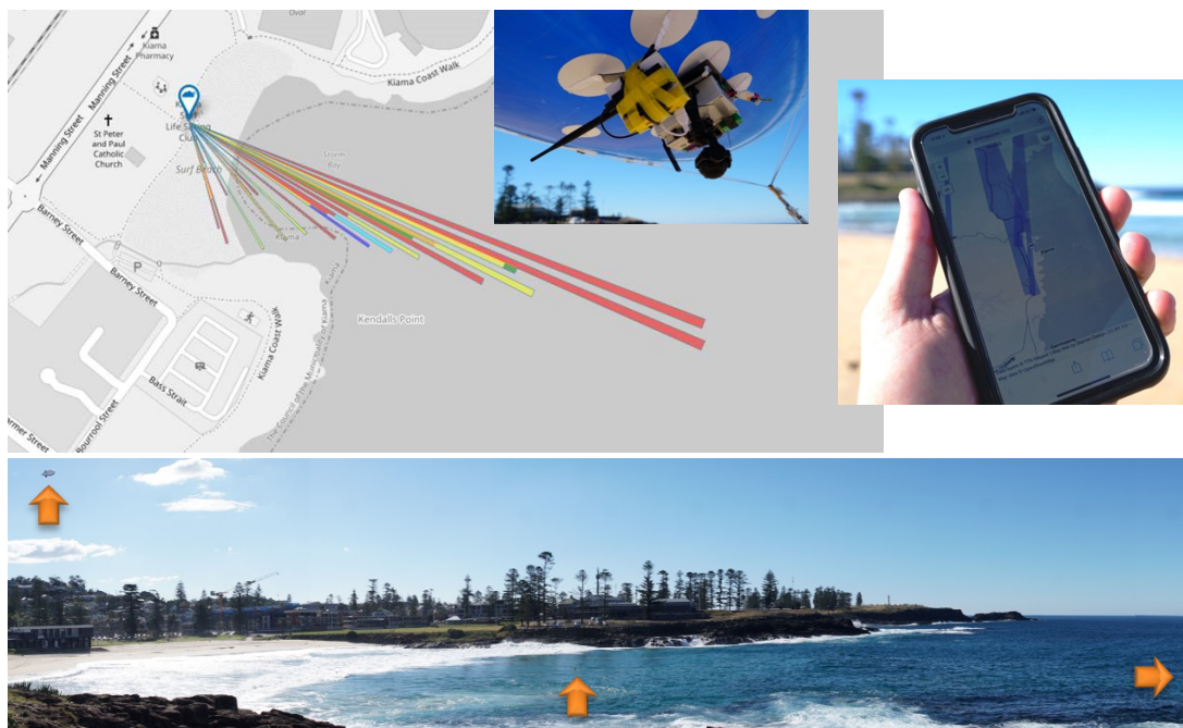
Figure 8. Top Left: IoT Tracking on the Things Network. Top Middle: the IoT Gateway packaged with battery and secured to the blimp. Top Right: Live view of the Gateway launched on the blimp connected to the network during testing at Kiama. Bottom: Landscape view of tracking area. Blimp can be seen at the upper left part of the picture (arrowed)—the small dot in the middle is a lifeguard on a paddleboard with the beacon (arrowed). Tracking was achieved out to a shark sonar buoy ~1 km offshore.
