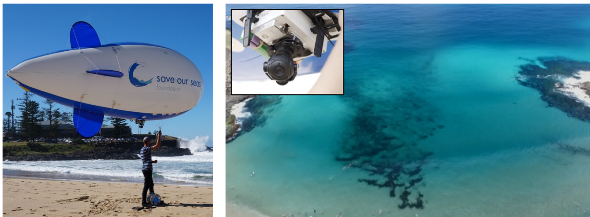
Figure 1. Left: Image of the inflated blimp, Project Aerial Inflatable Remote Shark–Human Interaction Prevention (Project AIRSHIP), with ground crew and tether at Kiama Surf Beach, NSW (May 2018). Right: Typical view from the blimp camera over Kiama. Inset: the image collection system with power supply, camera on gimbal, communication system, and custom mounting. The system allows for operators on the beach to control direction and zoom on the camera. Once in the air, the video feed is passed to computers at the beach.
