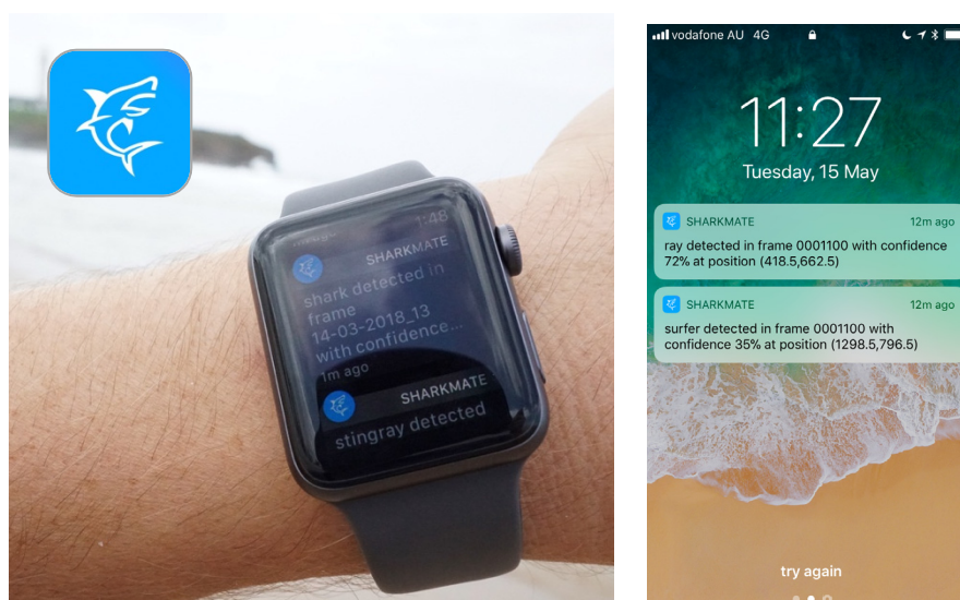
Figure 5. Examples of user interface (UI) image of the Sharkmate App Alerts on watch and on smartphone. The measure ‘confidence danger’ was a gauge how confident the detection of the Deep Learning neural network was for the detection event observed.
