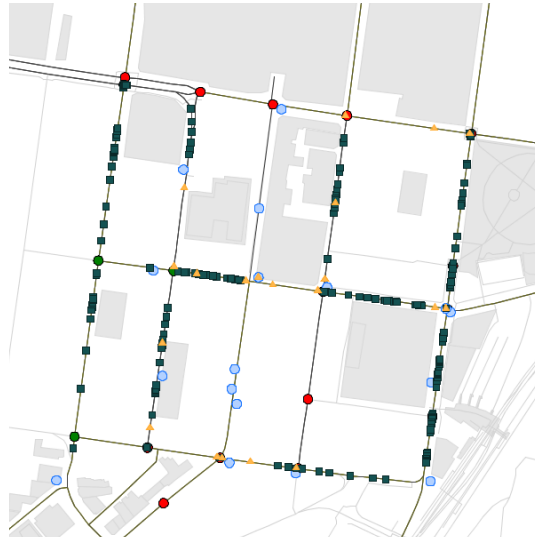
Fig. 5: Traffic Network. The red and green circles depict the traffic lights, whereas the blue circles represent the visual sensors. The blue squares represent the vehicles, the yellow triangles illustrate the pedestrians.
