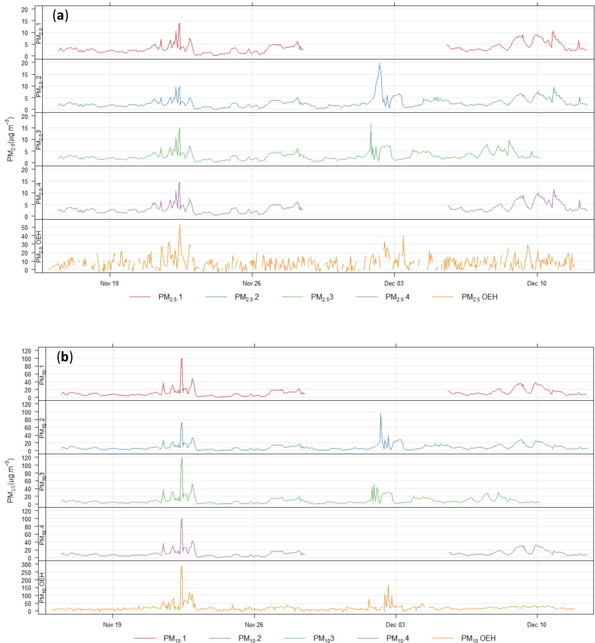
Fig 5. Hourly averaged PM measurements ( \mu\text{g m}^{-3} , note different scales) from 4 devices co-located with Department of Planning, Industry and Environment (DPIE) reference instrument in December 2018. (a) \text{PM}_{2.5} 1–4, \text{PM}_{2.5} DPIE and (b) \text{PM}_{10} 1–4, \text{PM}_{10} DPIE; at DPIE air quality monitoring station in Campbelltown, western Sydney. Missing data in plots 1 & 4 due to power failure, time lag in 3 from early December due to a failing battery in the device's clock.
