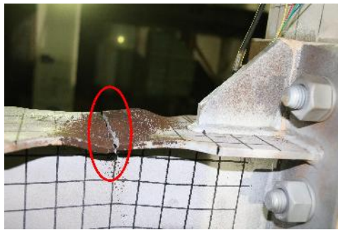
(b) Flange fracture at 0.05 rad
