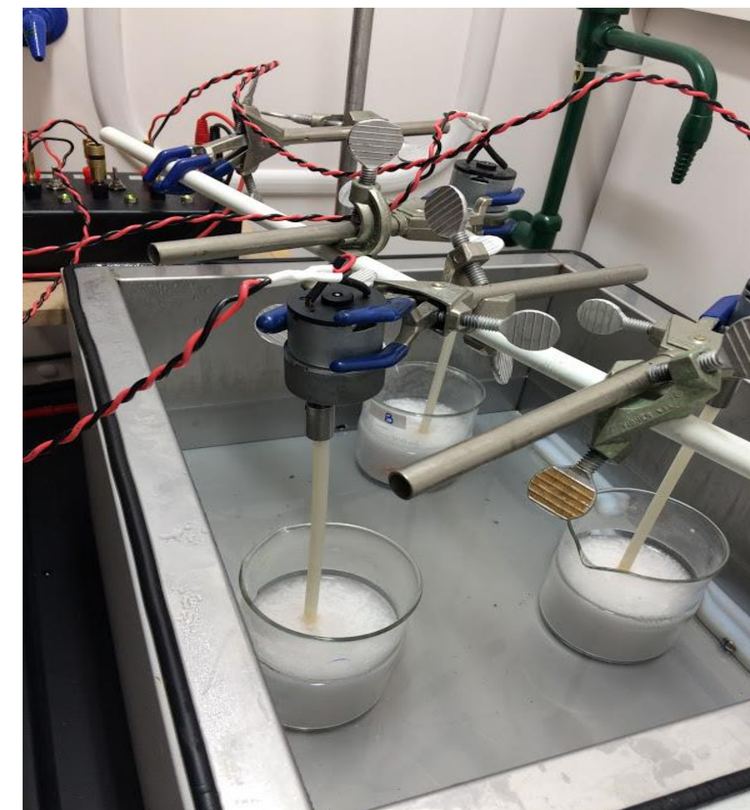
Fig 1. Water bath with rotating agitators used for starch digestion
