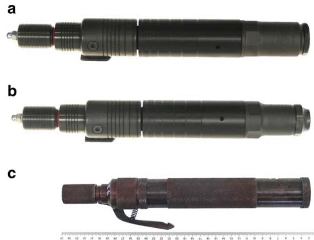
Fig. 2 The captive-bolt guns used for the test shots. a Make Schermer KR. b Make Schermer KS. c Make Pfeiffer
