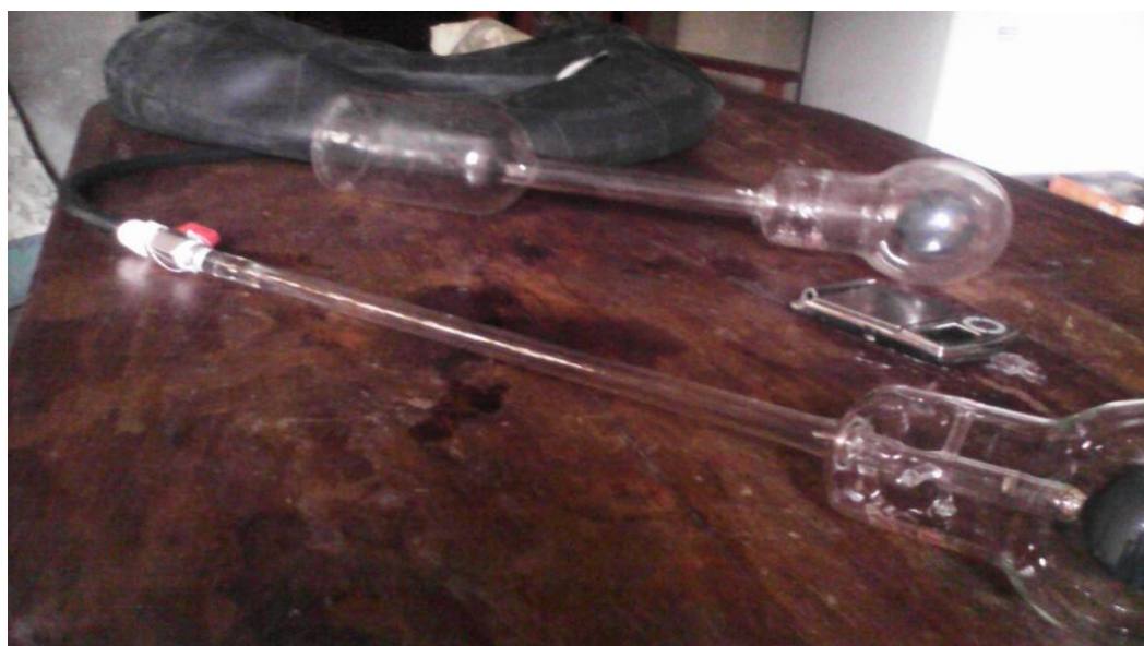
Figure 1. Pascal manometric tube used for gas analysis.
