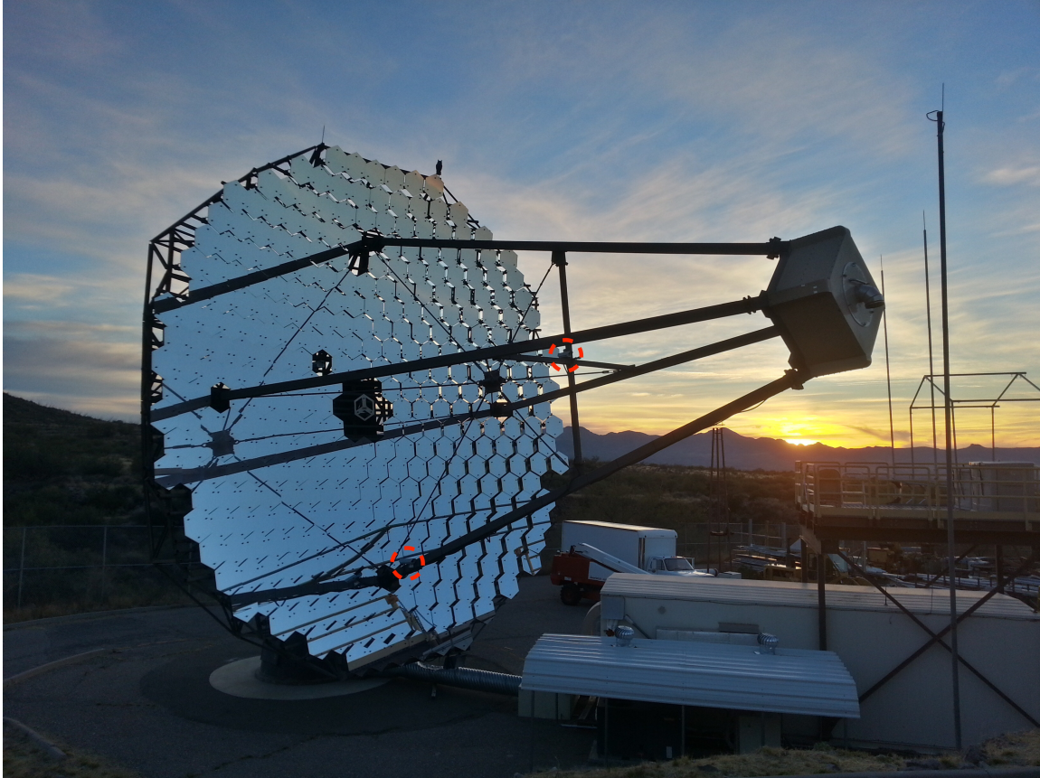
Figure 4.2: View of the 345 mirrors, the camera support structure, and the PMT camera housing at the end of the four supporting arms.
