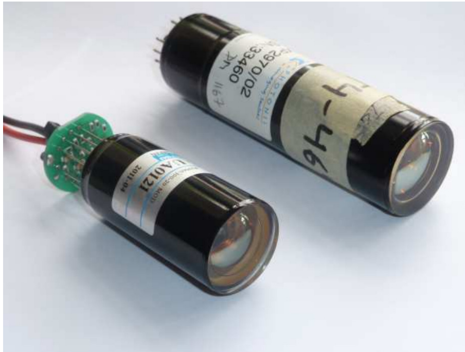
Figure 4.6: The two PMT models used in the VERITAS cameras [177].
