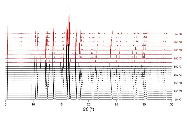
Figure 2: A plot of the PXRD experimental patterns of  $Fe_2As$  sample upon heating and cooling.
