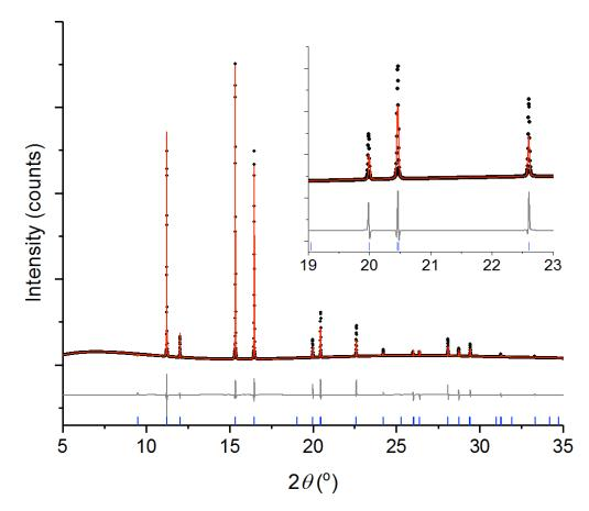
Figure 5: Final Rietveld refinement plot of the high temperature FeAs phase. The observed (black), calculated (red) and difference (grey) patterns, and peak marks for a new phase are shown. The observed pattern has been obtained by fitting the triplet unidentified peaks of the data obtained at 800C with single Pseudo-Voigt peaks.
