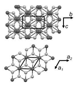
Figure 7: Crystal structures of FeAs phases: MnP-type (top) projected along the a axis and NiAs-type (bottom) projected along the c axis. As atoms and Fe atoms are light grey and dark grey, respectively.
