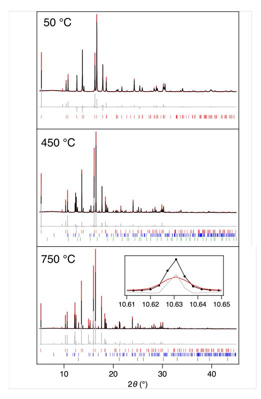
Figure 3: Rietveld refinement of the PXRD patterns of  $Fe_2As$ . The experimental (black), calculated (red) and difference (grey) curves are shown. Peak marks: red -  $Fe_2As$ , blue - FeAs, green -  $Fe_3O_4$ , and black - FeO.
