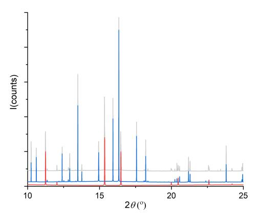
Figure 6: Synthetic pattern (red curve), experimental pattern (grey curve) of  $Fe_2As$  at 800 °C, and relative calculated pattern (blue curve) from the Rietveld refinement (including fayalite). Curves have been displaced vertically to aid observation.
