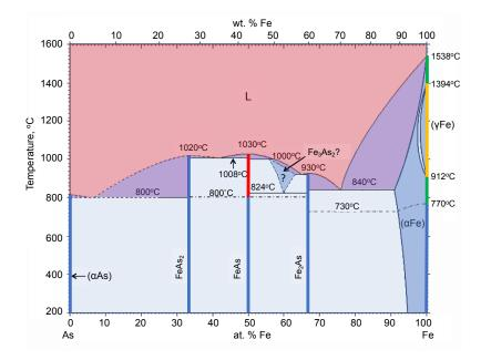
Figure 1: Phase diagram of the Fe-As system adapted from Okamoto<sup>2</sup>. Line phases are shown dark blue at room temperature and alternatively colored where polymorphs occur at high temperature. The postulated stability field of the  $Fe_3As_2$  phase is indicated.
