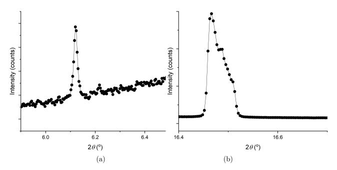
Figure 4: Example of parts of the diffraction patterns of our sample at 800 °C: (a) single peak, (b) triplet peaks.
