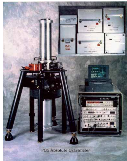
FIGURE 11.6. Absolute gravimeter of type FG5. Figure United States National Oceanic and Atmospheric Administration.
