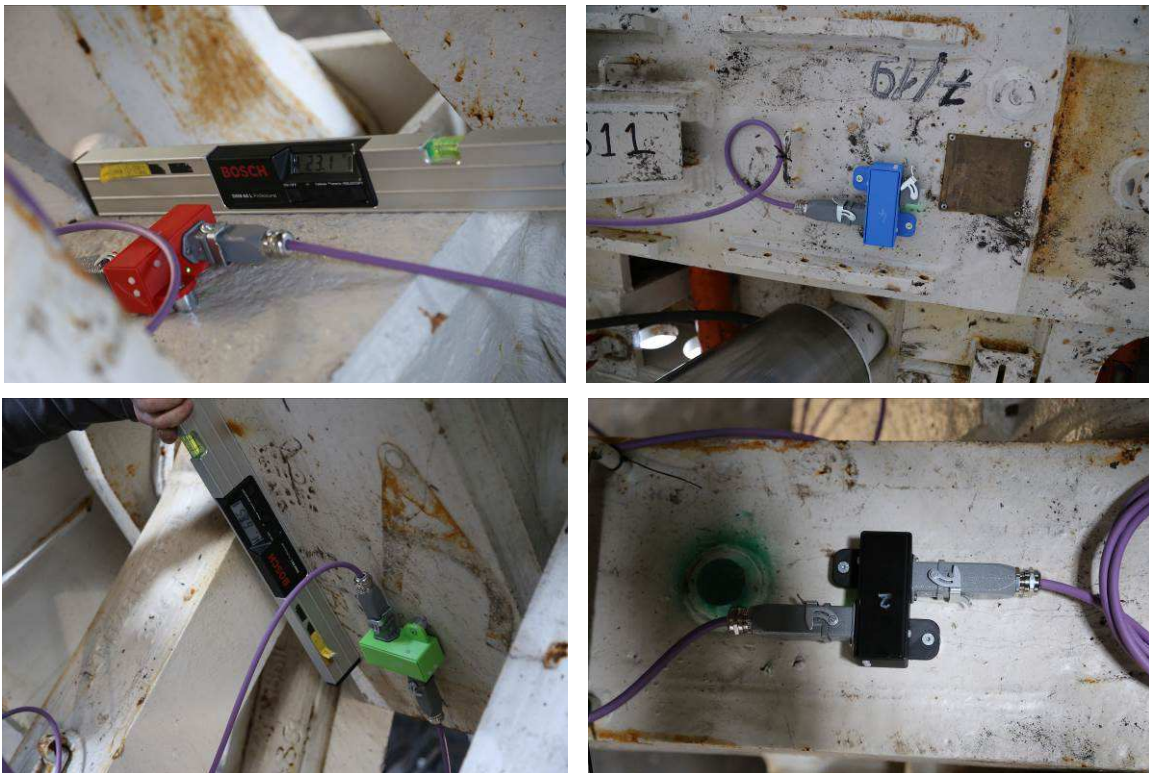
Fig. 8. Model of SSMS-I inclinometers: a) on the base, b) on the canopy, c) on the goaf shield, d) on the lemniscate linkage
