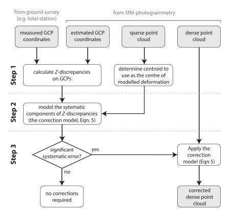
FIGURE 4. Summary workflow for detection and removal of modelled systematic topographic error from SfM surveys.
