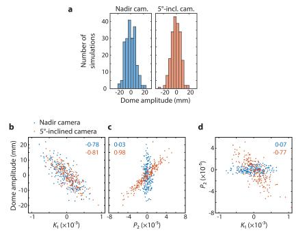
**FIGURE 8.** Distributions of doming amplitude and associated camera parameter values from survey simulations (Table 1) processed in PhotoScan, with  $P_2$  estimated. Surveys used either a nadir-pointing camera (blue) or a camera inclined at 5° (red) in pitch. Distributions of doming amplitude (a), and correlations between (b) doming amplitude and  $K_1$ , (c) doming amplitude and  $P_2$ , and (d) between  $K_1$  and  $P_2$  values. [Colour figure can be viewed at wileyonlinelibrary.com]
