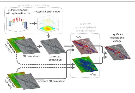
FIGURE 5. Workflow for using systematic topographic error removal to enhance precision-based change detection. [Colour figure can be viewed at wileyonlinelibrary.com]
