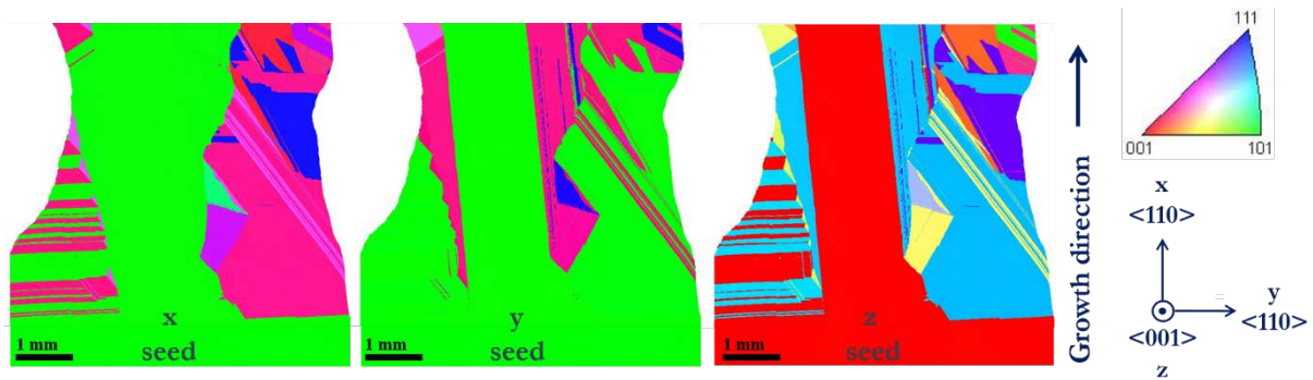
Fig. 2: Crystallographic orientation maps (IPF) of the solidified sample in the x (growth direction), y and z-directions obtained by EBSD ex situ measurements ( 7 \mu\text{m} step size) after the 13 th melting-solidification cycle performed with an applied temperature gradient G = 30 \text{ K/cm} and a cooling R = -0.2 \text{ K/min} .
