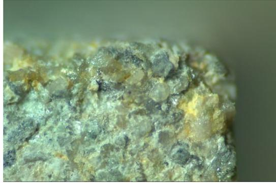
Figure 2. A corner of the rock probe, in the final setup configuration that gives the best image texture to calculate movements by DIC.
