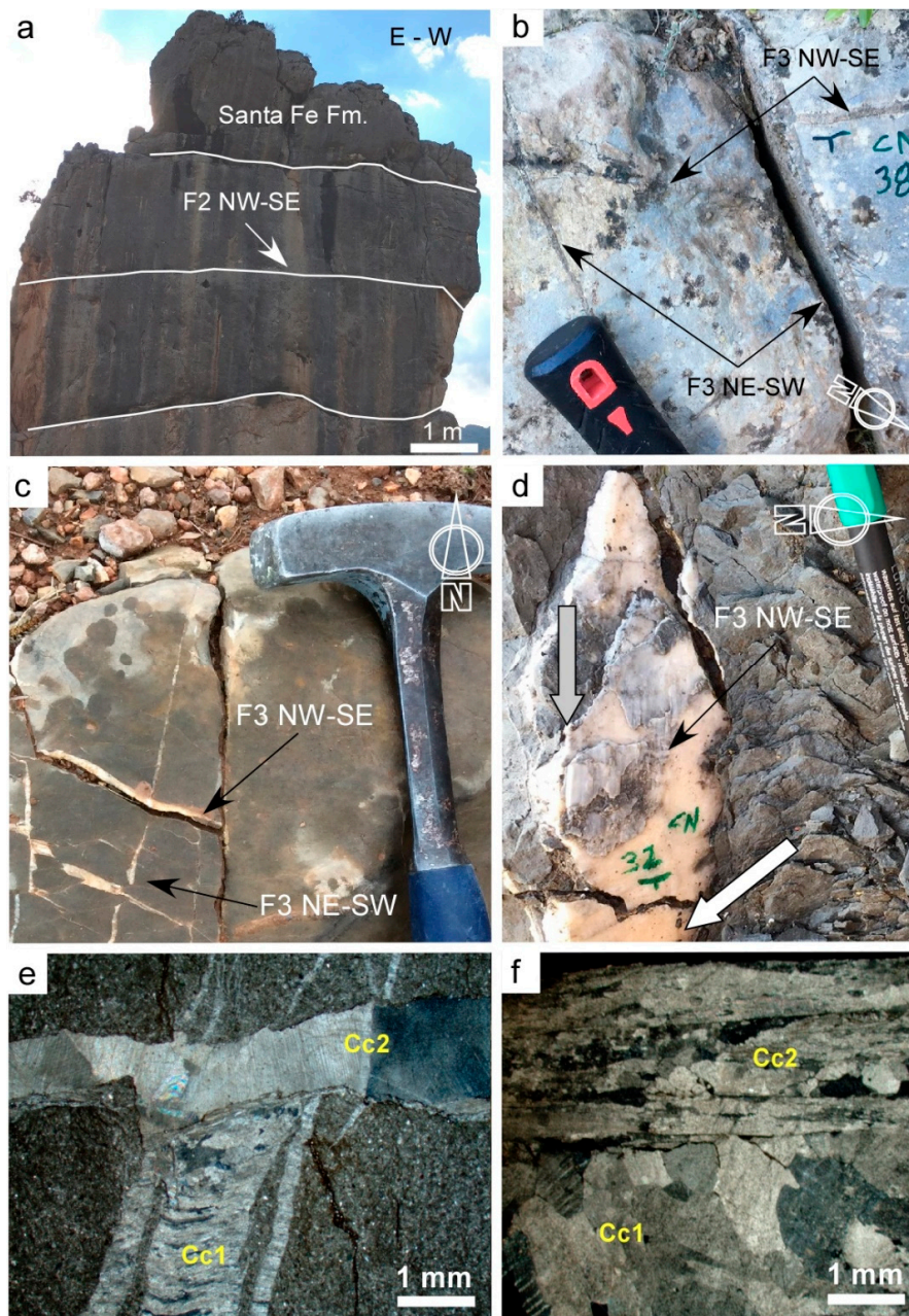
Figure 8. (a) F2: NW-SE non-mineralized fractures in the Santa Fe Formation. (b,c) F3: NW-SE and NE-SW conjugate fracture set. (d) F3 fracture showing a later reactivation with strike-slip movement (white arrow) and dip-slip movement (grey arrow). (e,f) Crosscutting relationship between calcite cements Cc1 and Cc2 (sample CN12). Cc2 clearly crosscuts and postdates Cc1 in F3 conjugate joints.
