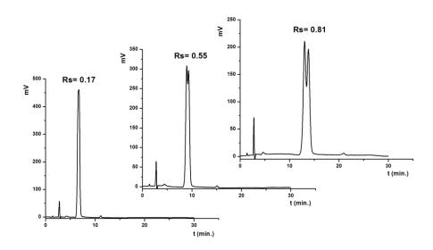
**Figure 2.** Superimposed chromatograms of partially overlapped profiles of *S:R* 95:5 ketoprofen. Chromatographic conditions as in Figure 1. Eluent compositions: see Table 3.
