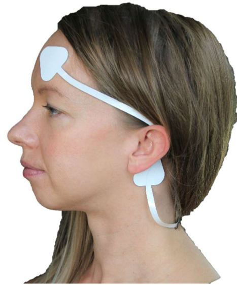
FIGURE 3. The test electrode sets, worn by one of the authors (L.K.) are positioned on the forehead and behind the ear (mastoid). The electrode sets based on the inks of the other manufacturer are attached to the corresponding location on the opposite side of the head.
