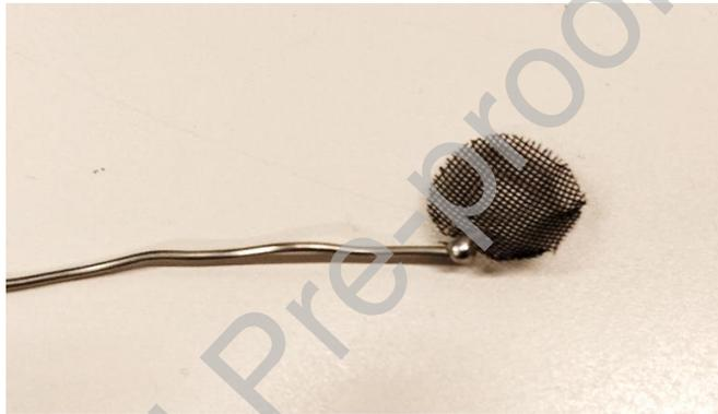
Fig. 5: Mesh “spoon” for sample insertion
