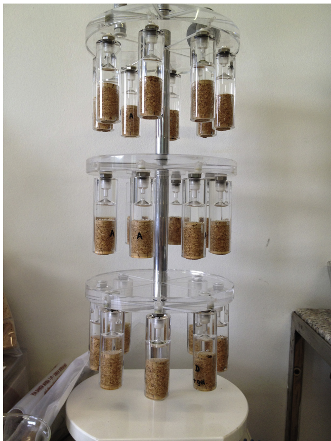
Fig. 1. Metalomecanica JAV instrument with the screwed bottle-neck shaped tubes. The cork stoppers and the synthetic wine solution are visible.
