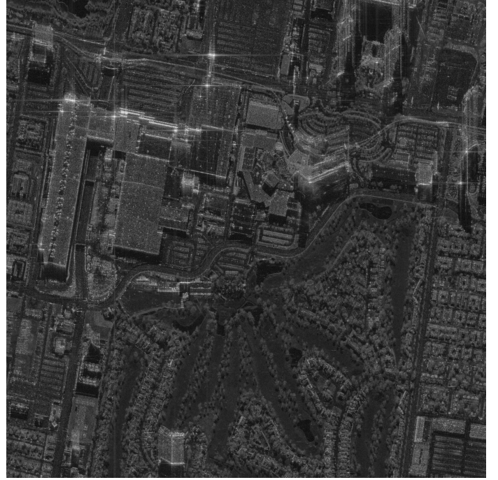
Fig. 6. The study area of Las Vegas shown by the mean amplitude (log scale) of a TerraSAR-X InSAR stack.
