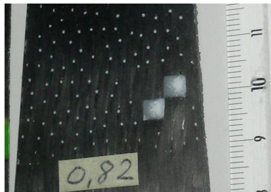
Figure 21: Composite specimen with correlation pattern and marker applied within the manufacturing process.
