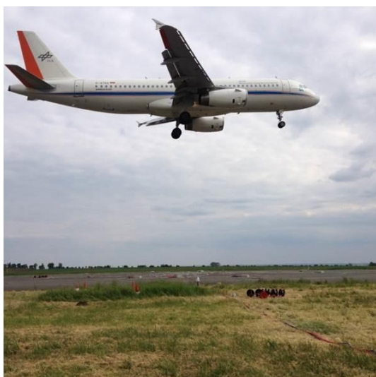
Figure 15: The DLR ATRA passing over a microphone array (Photo: DLR).
