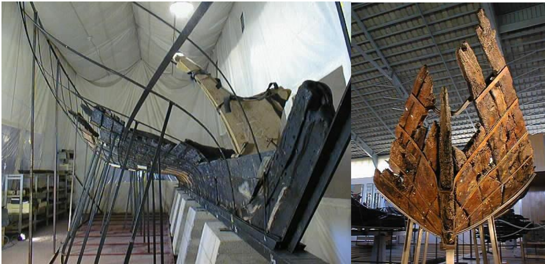
Figs. 31 and 32: Marsala 1 by comparison to Fiumicino 5 . The keel is considerably deeper in the former.
