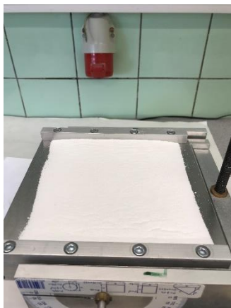
Figure 3 - Method for evaluating the angle of slide described as fine layer method.
