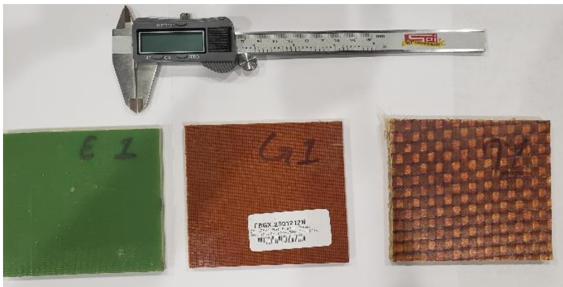
Fig 2. Sample Specimens for High Temperature G-11 (left), Economical Garolite (middle) and Impact Resistance Garolite (right)
