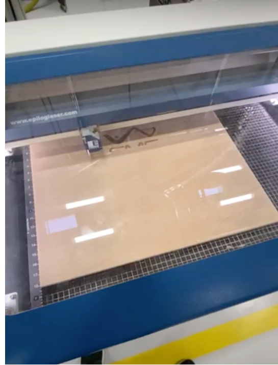
Figure 34: Laser Engraving in Progress
