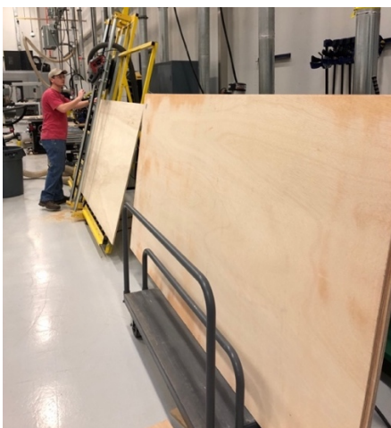
Figure 16: Plywood Loading and Cutting
