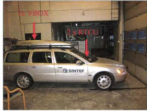
Figure 2 Placement of antennas on test vehicle
