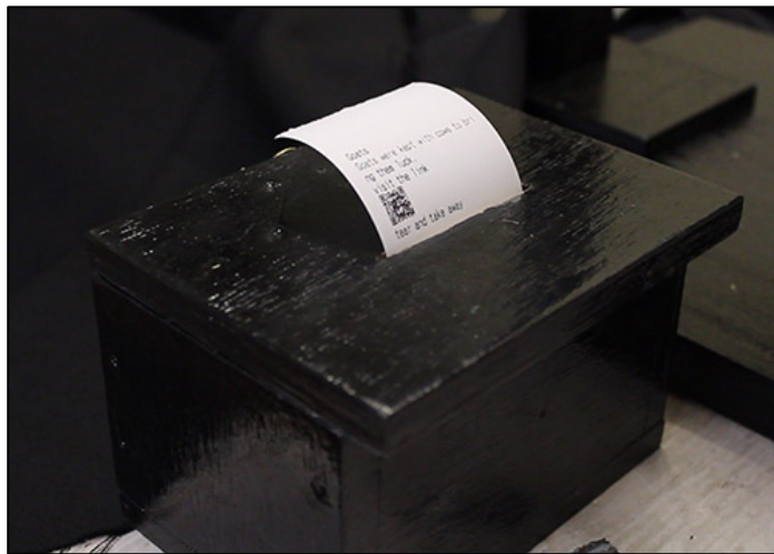
Figure 5.8 A thermal printer, which printed receipts, was introduced to the design to replace the screen.
