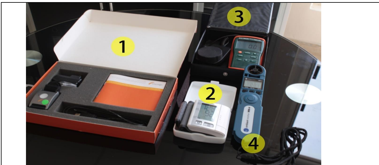
Fig. 5 The devices used in physiological and environmental measurements (1) Affectiva Q Sensor (2) Heart Rate monitor (3) illuminance monitor (4) The weather station.
