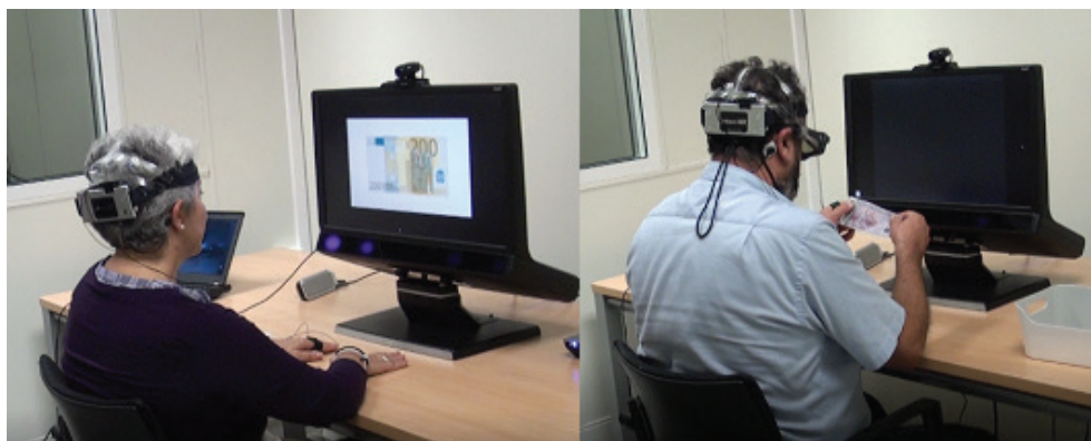
Picture 1. Left: Person completing first phase with TOBII TX300. Right: Person completing second phase with SMI glasses.
