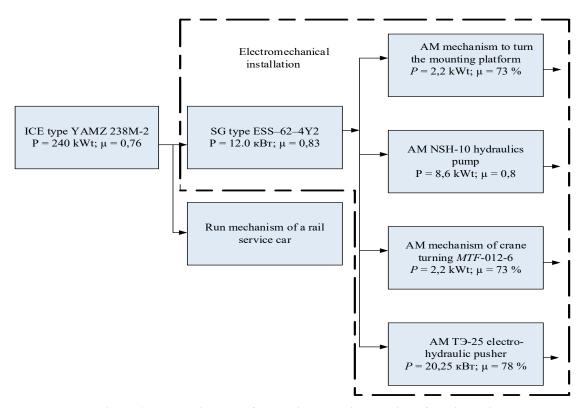
Figure 1 - Block diagram of the main power installation of a rail service car.
