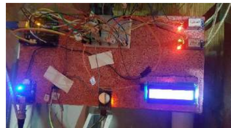
Gambar 7. Prototype rangkaian peyiraman otomatis
