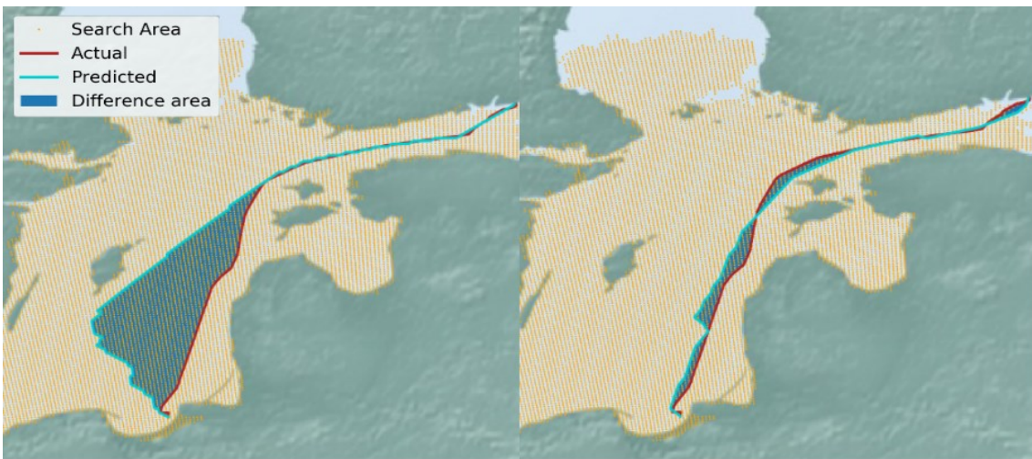
Figure 21. Summer route prediction results visualized using the adjacent model (left) and the ship model (right). Tile size is 5 km x 5 km. Voyage id in the validation set is 5672.
