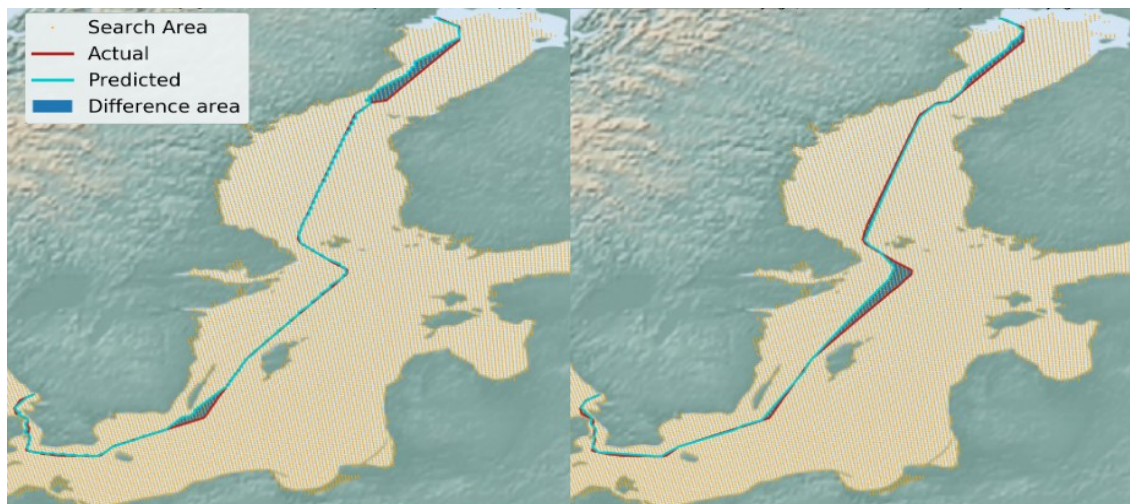
Figure 19. Summer route prediction results visualized using the adjacent model (left) and the ship model (right). Tile size 5 km x 5 km. Voyage id in the validation set 802.
