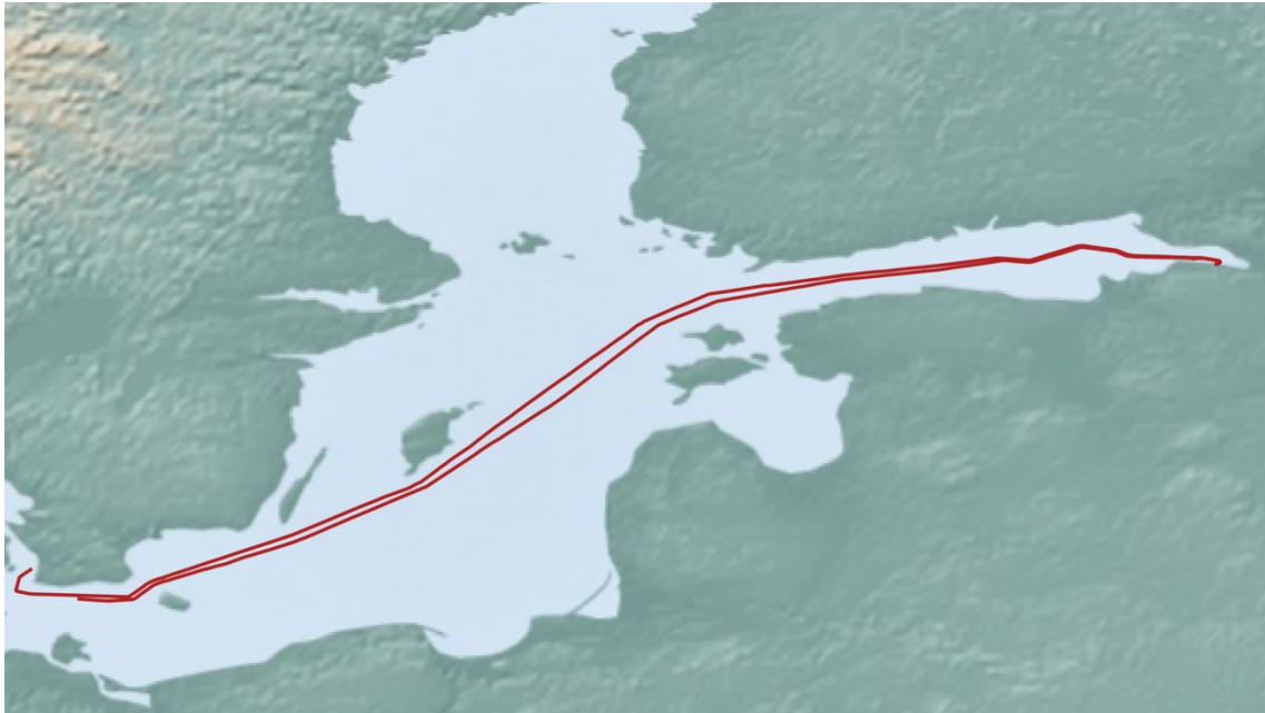
Figure 14. An incorrectly calculated voyage. The calculation failed to detect the port visit of the vessel in the east which resulted in the addition of the return trip to the voyage.
