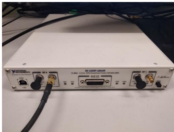
Figure 7. USRP model 2954R used for recording the signal.
