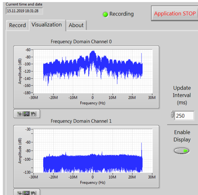
Figure 11. Frequency spectrum of channel 0 and 1 of the Labview interface.
