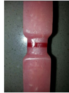
Figure 1. Acrylic specimens with 3mm wax in its narrowest part
