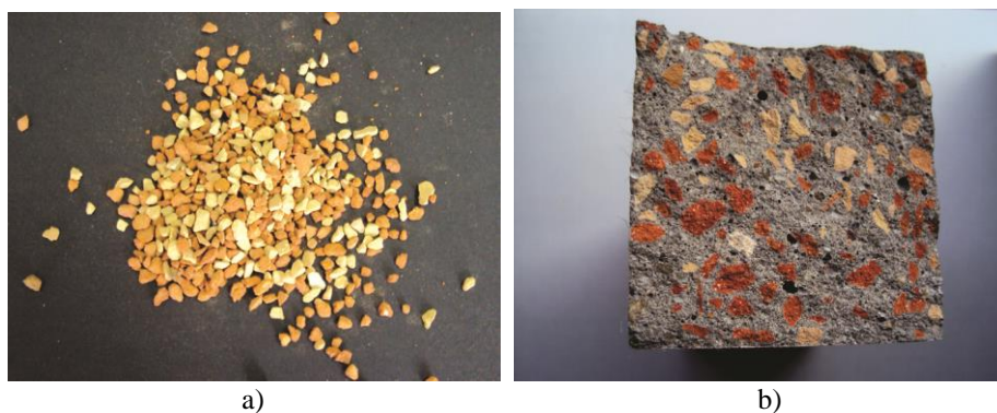
Fig. 1 Used materials: a) recycled crushed brick aggregate 2/4 mm, b) section of the mortar sample with recycled crushed brick as aggregate
