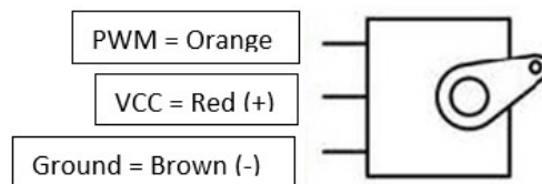
Figure 2. Arms of the Servo Motor
