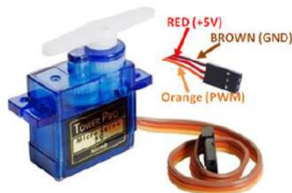
Figure 1. Servo Motor Pinout Wires
