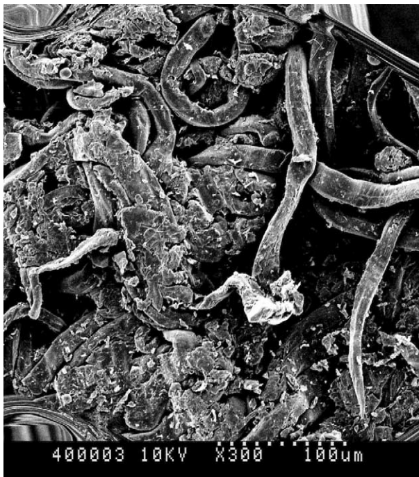
Figure 5 Scanning electron microscopy images of lignin fusion band on the bondline with cellulose fibers and wood cells (tracheids) immersed in it obtained during welding at magnification 300 \times showing general appearance of the band.
