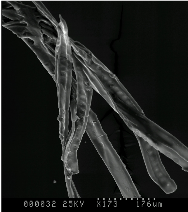
Fig. 7. Treated pine sapwood whose tracheids are easily manually disjoined. Softening and darkening are strongly related and both phenomenons imply a lignin modification.
