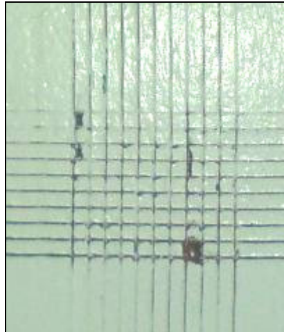
Fig. 13. Cross-cut testing carried out on aqueous based coating applied on densified composite
