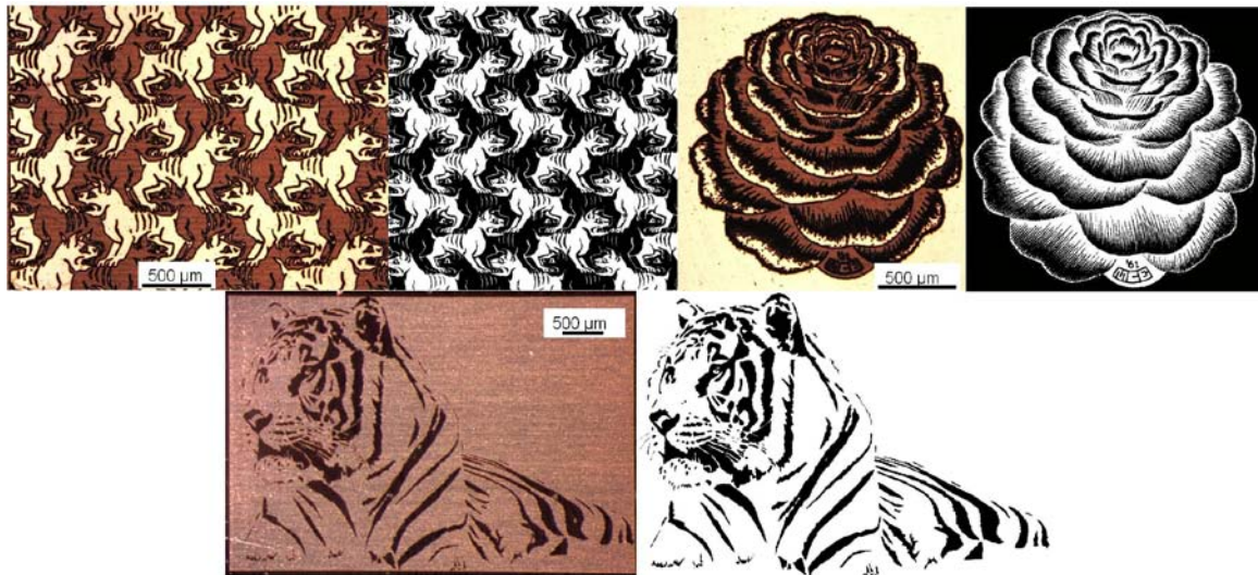
Figure 11: Structures based on black-and-white images: comparison of the original picture and the microscope image, 120 mW, 300 kHz, 3 µm pitch, 30 layers 15, 16, 17
