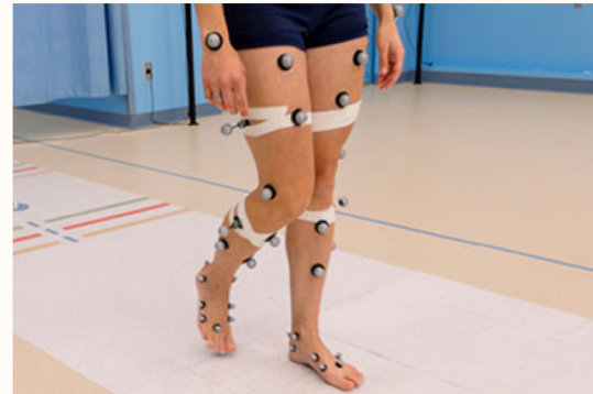
Figure 2. Approximation of motion capture receptor placement on the lower limb of a subject (Mayo Clinic)
