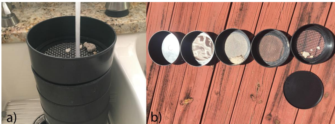
Figure 7. a) Stacked sieves for fossil retention, b) Sieves for fossil sorting. Sizes are arranged from right to left: 5, 10, 60, 230.
