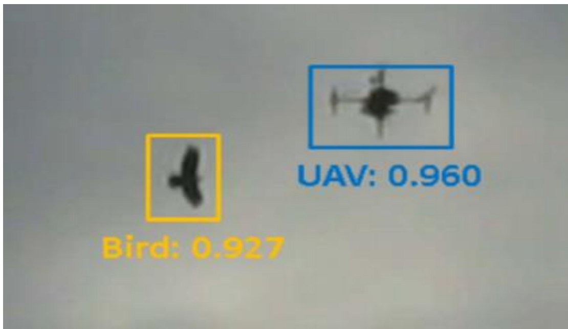
Fig. 2. Flying object detections can be filtered by a classifier to reduce the number of false alarms Source: [36].
