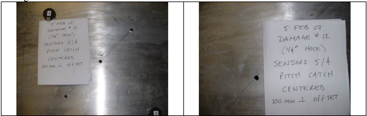
Pitch-Catch (5 to 4): 35 kHz Far Sensor (4)
