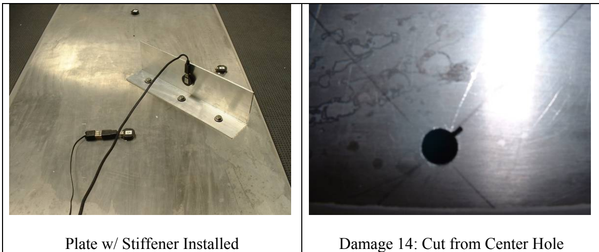
Figure 4.12: Damage Testing w/ Stiffener Installed
